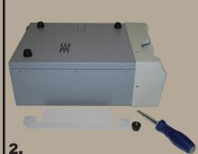
Carefully remove two of the rubber feet on one side of the ViroVac.
